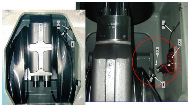
1. Wireless temp sensor; 2. Antenna; 3. Bracket; 4. Antenna Cable
